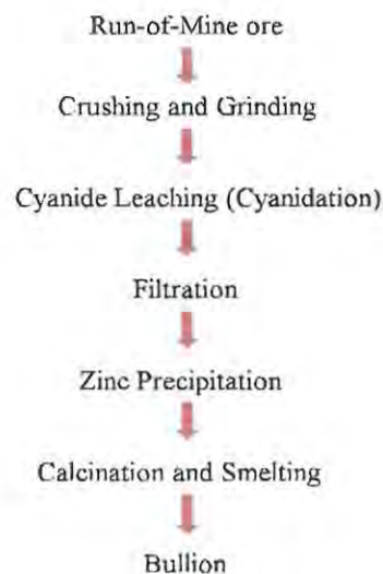
Figure 1.4: Essential steps involved in the cyanide-based extraction process (Woodhouse, 1986).
