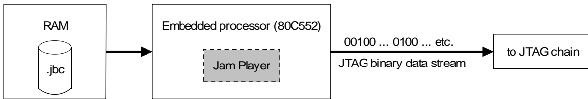
Figure 7.18 Block diagram of ISP using a Jam file and Jam Player (Adapted from Embedded programming using the 8051 & Jam byte-code, p.4).
