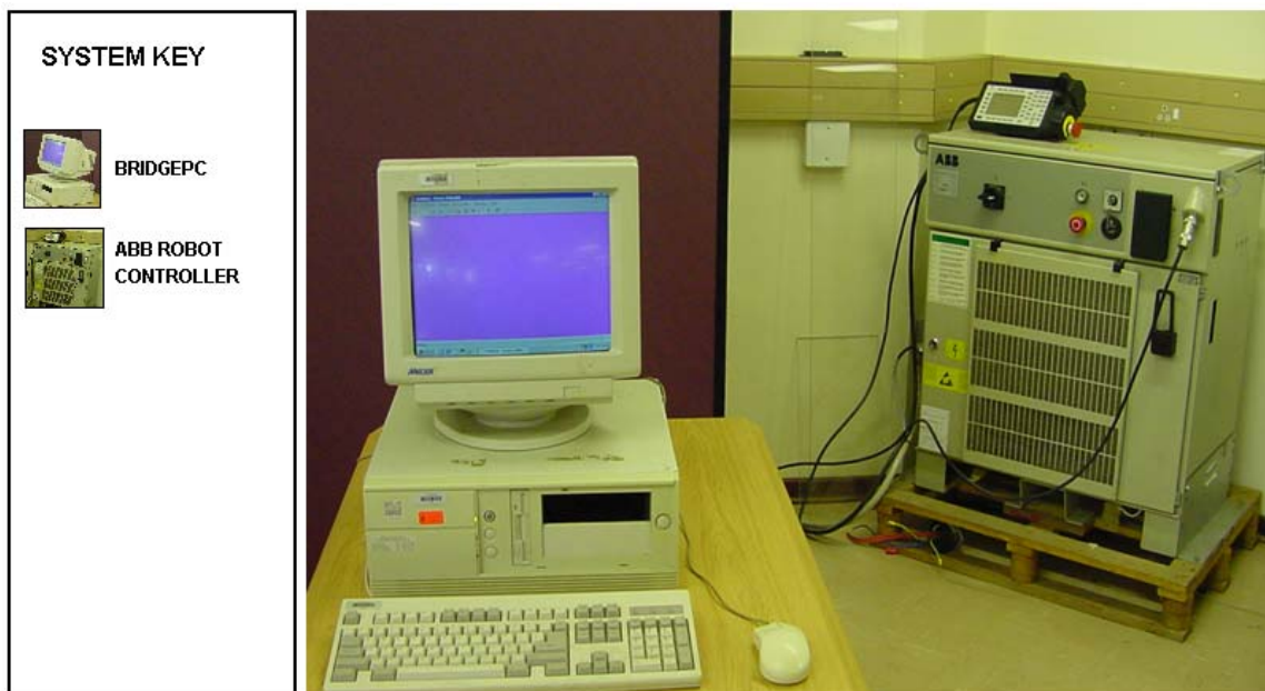
Figure 3.2b: 1400 ABB Robot Controller & Bridge PC – System Setup
