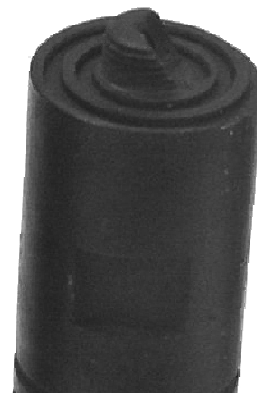
Figure 2.6: Examples of various tool pin profiles used for the FSW process at the Port Elizabeth Technikon
