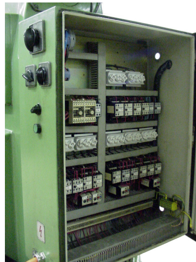
Figure 3.3: Control panel mounted on back of machine before redesign
