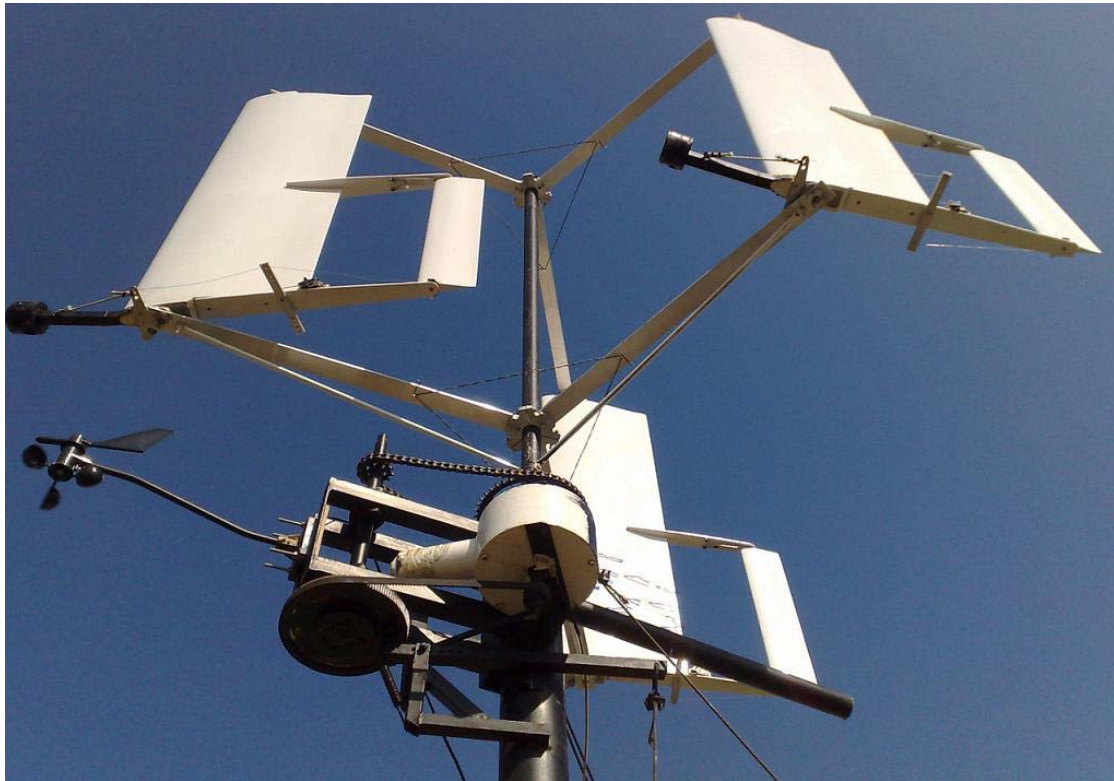
Figure 6.10 Control arms at max power setting – unit rotating under load
