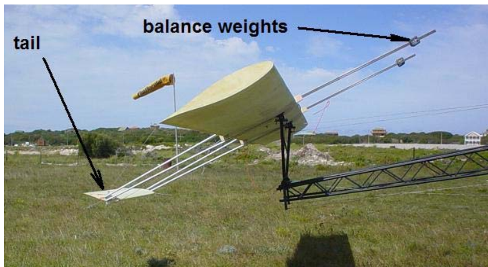
Figure 3.4 Horizontal aerofoil on hinged arm-indirectly controlled
