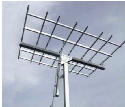
Figure 3.2: Example of a Basic Mounting Structure with Tracker
