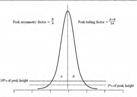
Figure 3.3 Schematic representation for the determination of peak asymmetry and peak tailing factors
