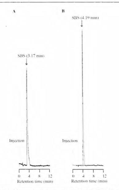
Figure 3.2 Representative chromatograms developed using USP [95] (A) or BP [23] (B) chromatographic conditions
