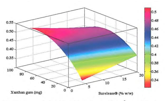
Figure 6.39 Response surface plot depicting the effect of xanthan gum and Surelease<sup>®</sup> on the mechanism of SBS release with Methocel<sup>®</sup> K100M and Carbopol<sup>®</sup> 974P concentrations at the centre level
