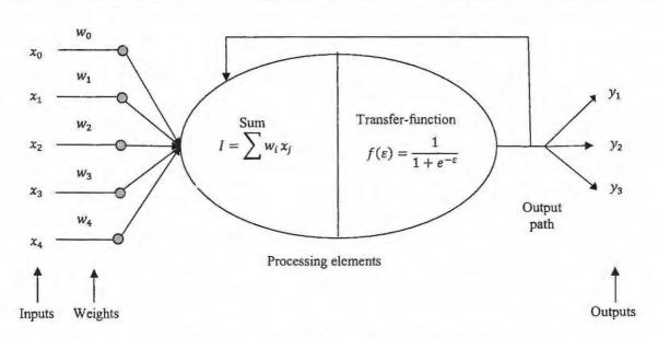
Figure 7.1 A simple artificial neuron, adapted from [209,211]
