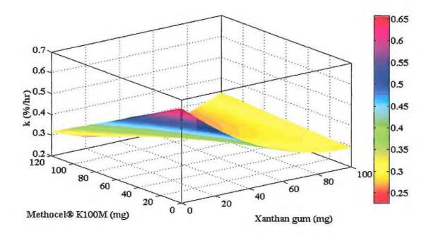
Figure 6.31 Response surface plot depicting the effect of Methocel<sup>®</sup> K100M and xanthan gum on SBS release rate with Carbopol<sup>®</sup> 974P and Surelease<sup>®</sup> concentration at the centre level
