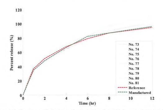
Figure 8.16 Dissolution profile simulation of hypothetical formulations 73-81 compared with the reference and manufactured formulations
