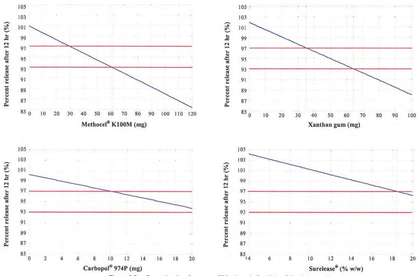
Figure 8.7 Constraint plots for percent SBS released after 12 hr of dissolution testing
