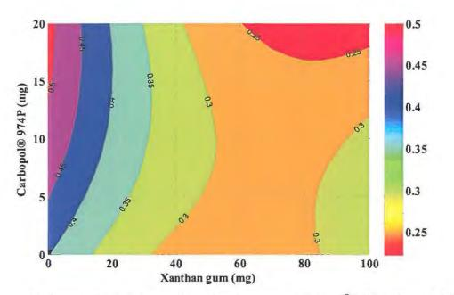
Figure 6.34 Contour plot depicting the effect of xanthan gum and Carbopol<sup>®</sup> 974P on the rate of SBS release with Methocel<sup>®</sup> K100M and Surelease<sup>®</sup> concentrations at the centre level
