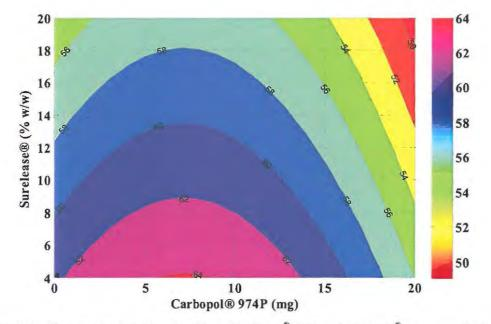
Figure 6.26 Contour plot depicting the effect of Carbopol<sup>®</sup> 974P and Surelease<sup>®</sup> on percent SBS released after 4 hr with Methocel<sup>®</sup> K100M and xanthan gum concentrations at the centre level
