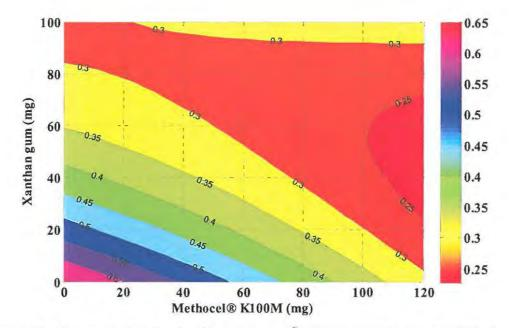
Figure 6.32 Contour plot depicting the effect of Methocel<sup>®</sup> K100M and xanthan gum on SBS release rate with Carbopol<sup>®</sup> 974P and Surelease<sup>®</sup> concentrations at the centre level
