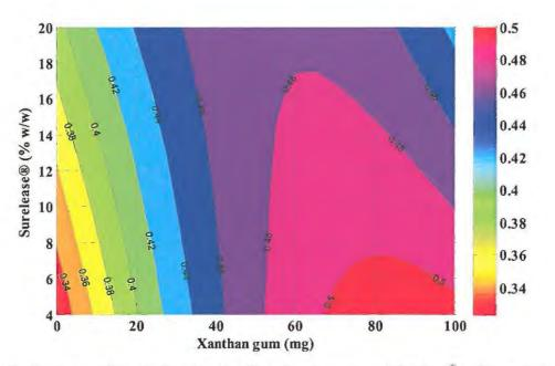
Figure 6.40 Response surface plot depicting the effect of xanthan gum and Surelease<sup>®</sup> on the mechanism of SBS release with Methocel<sup>®</sup> K100M and Carbopol<sup>®</sup> 974P concentrations at the centre level
