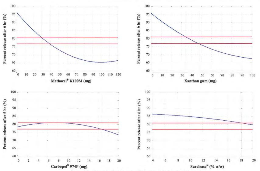
Figure 8.5 Constraint plots for percent SBS released after 6 hr dissolution testing
