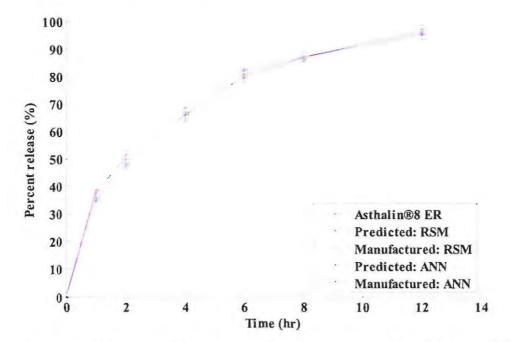
Comparison of formulations predicted and manufactured from RSM and ANN Figure 9.1 compared with the reference formulation
