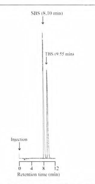
Figure 3.9 Representative chromatogram of SBS and TBS using the optimised mobile phase
