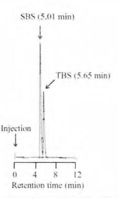
Figure 3.6 Typical chromatogram showing the separation of SBS and TBS using 20% v/v ACN in 18 mM phosphate buffer at pH 4, containing 15 mM sodium octane sulphonate
