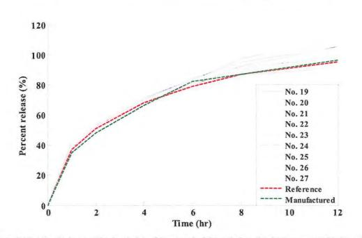
Figure 8.10 Dissolution profile simulation of hypothetical formulations 19–27 compared with the reference and manufactured formulations
