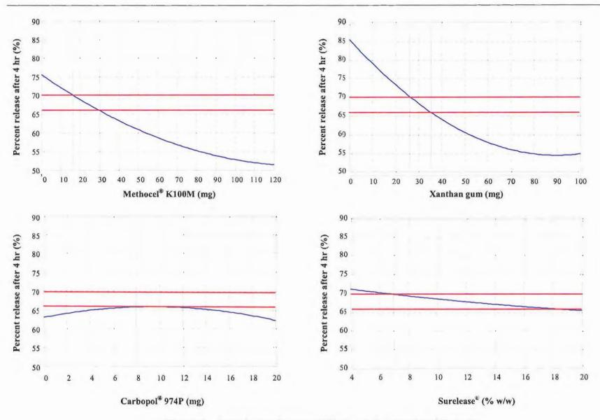
Figure 8.4 Constraint plots for percent SBS released after 4 hr of dissolution testing
