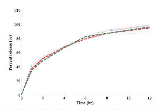
Figure 8.17 Dissolution profile simulations for formulations that are similar to the reference (red line) and manufactured (green line) formulations
