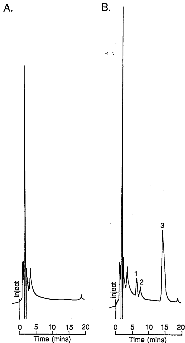
Figure 3.7 HPLC chromatograms of (A) blank human urine and (B) human urine spiked with (1) norcyclizine (8.01ng/ml), (2) cyclizine (8.22ng/ml) and 200ng/ml of (3) internal standard (chlorcyclizine).
