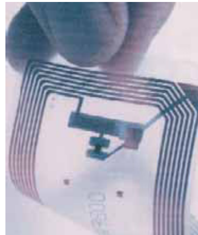
Figure 4: Sample of Passive RFID Tag (UPM Rafsec, 2006)
