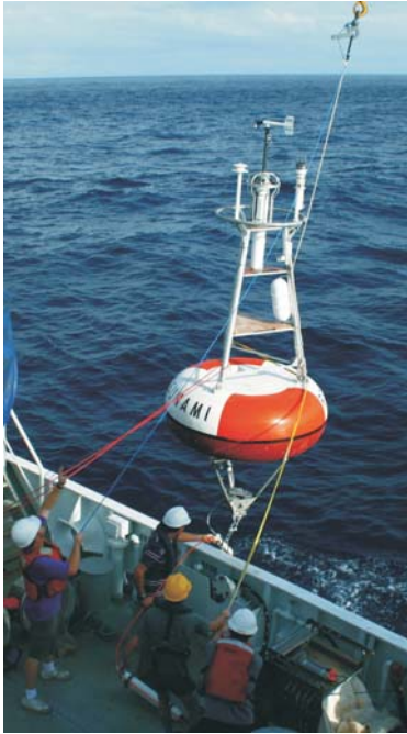
Fig. 4. An ATLAS deep-sea buoy being moored during an ASCLME cruise in 2008. This buoy boasts a large number of meteorological and oceanographic sensors, the readings of which are transmitted in real time.
