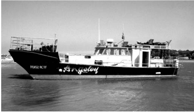
Fig. 1. The larger deckboat (18–25 m) vessel to be used in the octopus pot fishery.
