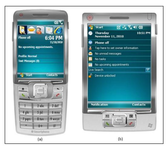
Figure 6.5: Windows Mobile SDK Emulator (a) Standard (b) Professional
