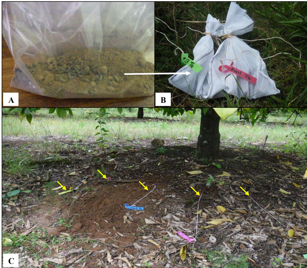
Figure 3.2: (A) 0.5 g of formulated product mixed with 100 g autoclaved soil; (B) labelled net bags containing formulated product prior to burial; net bags buried in the soil underneath the canopy of a citrus tree; (C) the location of the bag was identified by the string (string was attached to the bag) and the isolate was identified by the label. The yellow arrows indicate the location of the bags in the soil underneath the tree canopy.
