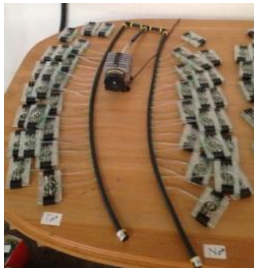
Figure 3.2 Series of 40 Munger cells of which half contain irradiated and half non-irradiated male FCM on treated leaf substrate connected to an air-flow system.
