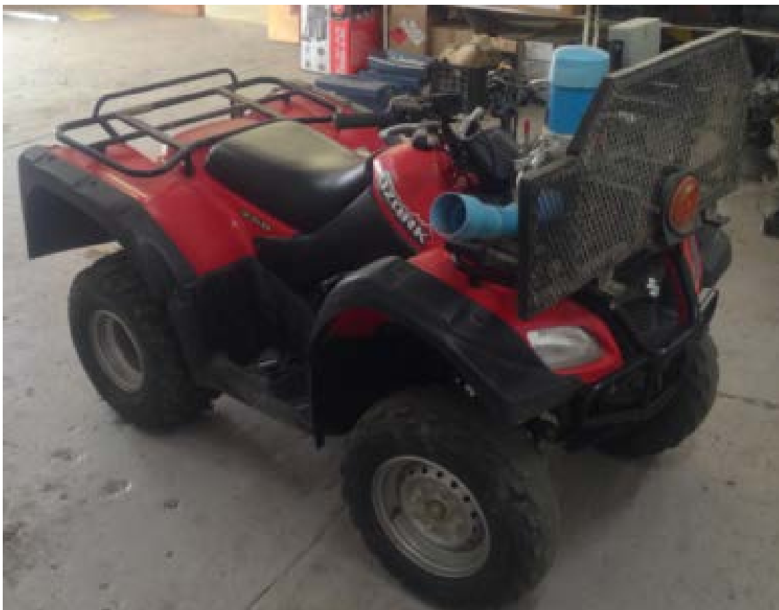
Figure 4.3 A specially equipped ATV used in the SIT programme for ground release of irradiated FCM in citrus orchards.
