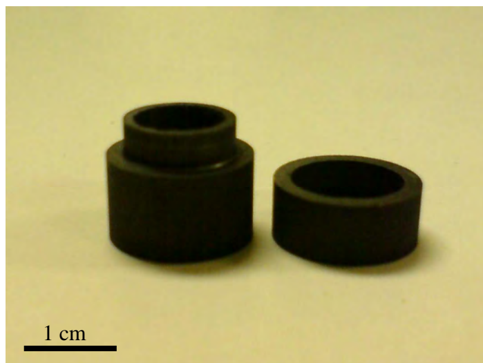
Fig. 5.4. Graphite specimen holder used to contain specimens during annealing in the Webb 89 furnace.
