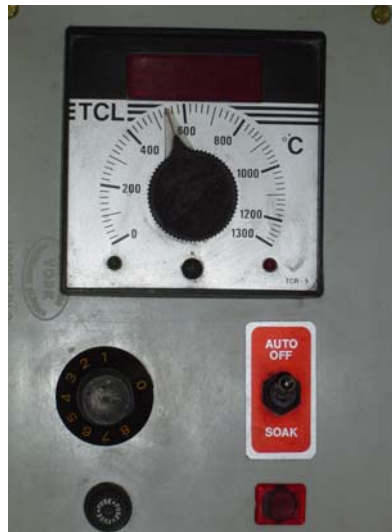
Figure 1.10 A photograph of an electric control instrument which is used to control the temperature of the kiln as well as having a soak control mode that allows the kiln temperature to be maintained at the upper temperature set or a specific firing.
