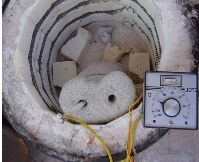
Figure 1.16 A photograph of a thermocouple inserted into a core prior to firing. The photograph shows the pyrometer which records the temperature of the thermocouple.
