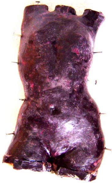
Figure 6.2 A photograph of the wax female torso 300 mm tall illustrating the core pins that were inserted into the wax prior to the core being poured into the hollow mould.
