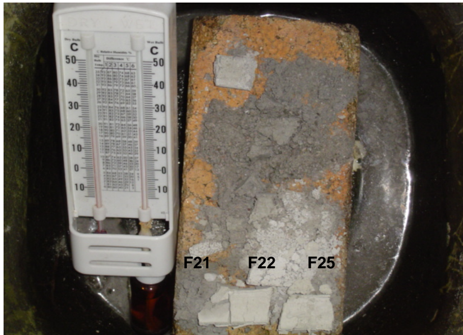
Figure 4.1 A photograph illustrating three naked test bars disintegrating inside the R H C apparatus.
