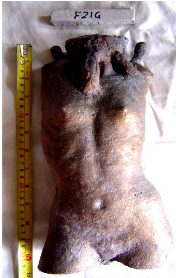
Figure 6.16 A photograph of the outer surface of the female torso (300 mm high) cast in bronze using formula F21G as the core body.
