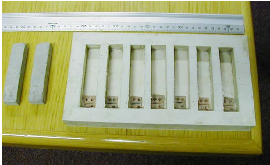
Figure 1.5 A photograph of the silicone rubber mould showing two naked test bars to the left of the photograph that have been removed from the mould.
