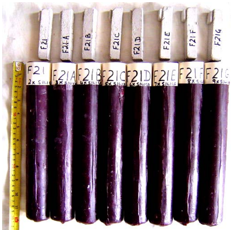
Figure 6.8 A photograph of one group of hollow wax tubes 300 mm x 30 mm with naked test bars as comparative controls having the same formulae that was poured into the corresponding wax tube.
