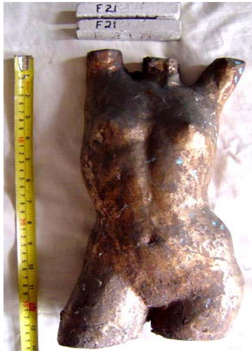
Figure 6.4 A photograph of the 300 mm bronze cast female torso that was filled with core formula F21.
