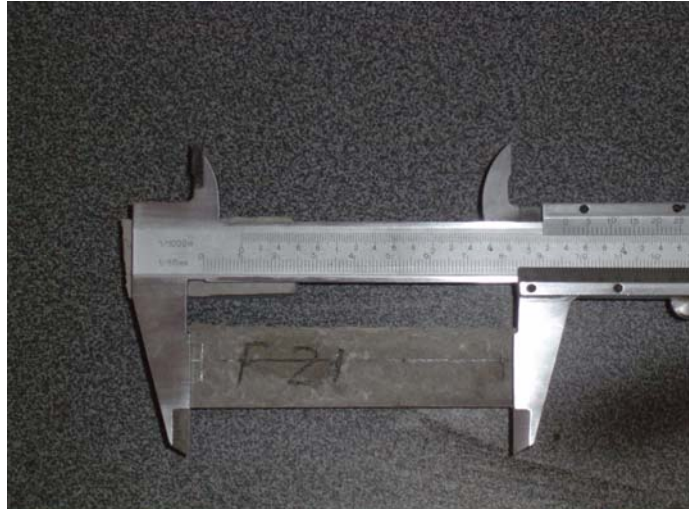
Figure 1.8 A photograph illustrating the vernier caliper, which will be used to measure a typical test bar in the test for shrinkage.
