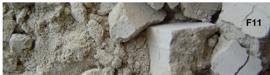
Figure 2.7 Formula 11 also broke into large soft powdery chunks when lightly touched after 72 hours.
