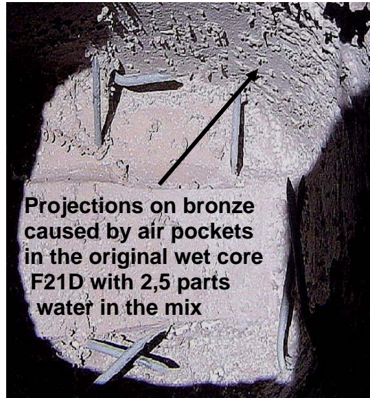
Figure 6.30 Internal view of figure 6.28
