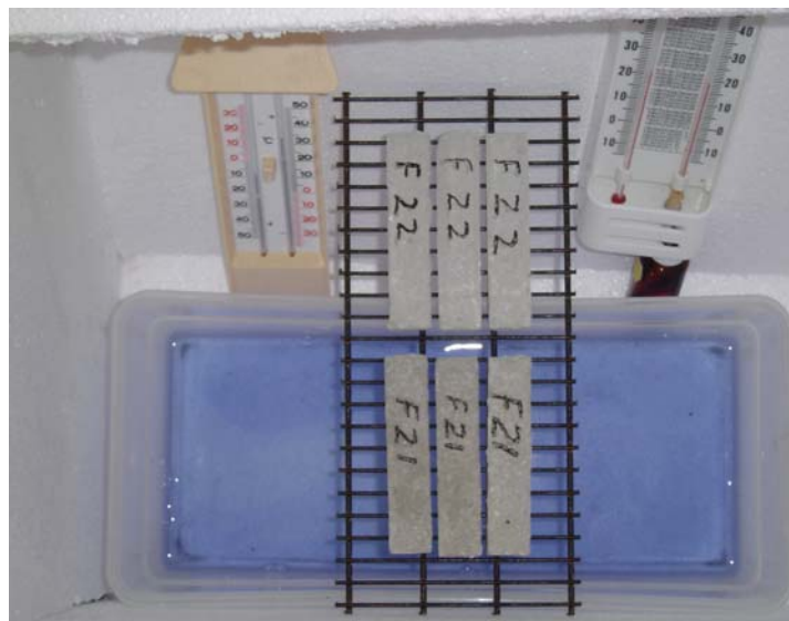
Figure 1.9 A photograph illustrating the interior of the R H C apparatus with dimensions of 400 mm x 400 mm x 400 mm. Naked test bars F21 and F22 (as examples) have been placed on the grid as illustrated, after first having been fired to either of 900°C, 945°C or 1000°C.
