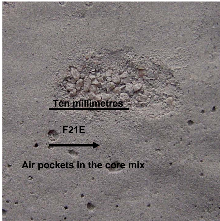
Figure 6.22 A photograph of the compacted surface of fired core formula F21E.
