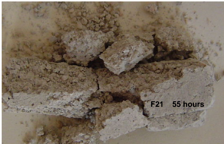
Figure 3.4 The sides of the naked test bar (F21) have fallen away from the main body after 55 hours.
