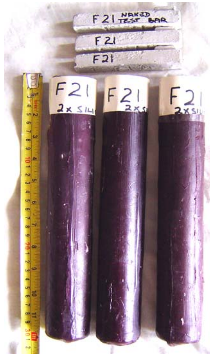
Figure 6.1 A photograph of three wax tubes 300 mm x 30 mm that were filled with core formula F21, invested in the ceramic shell and sintered with the three naked test bars depicted in the photograph before being cast in bronze.
