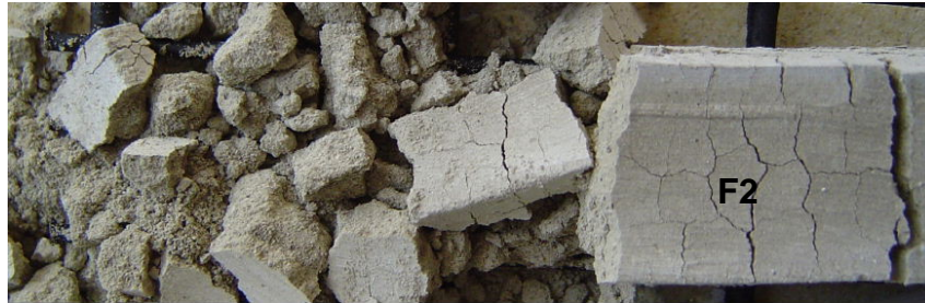
Figure 2.6 Formula F2 (pure cement) broken into large soft powdery chunks when lightly touched after 72 hours.
