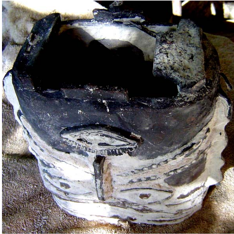
Figure 6.26 A photograph of the open-ended four-litre mask with the outside ceramic investment partially removed.
