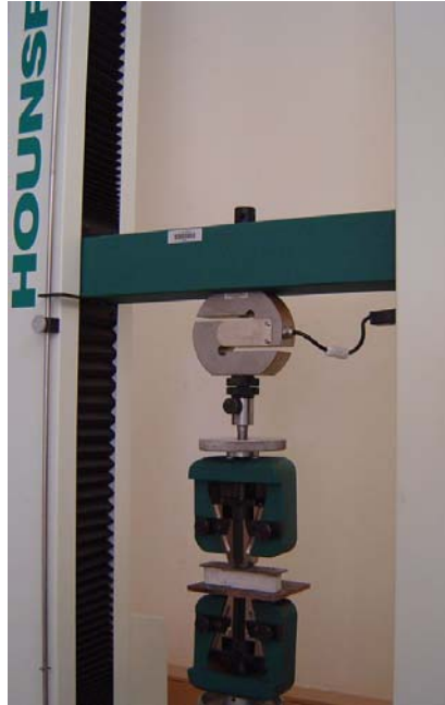
Figure 1.7 A photograph of the Hounsfield computerized test equipment. The photograph shows how a naked test bar made from a core formula will be tested for compressive strength, which is measured in megapascals (MPa).
