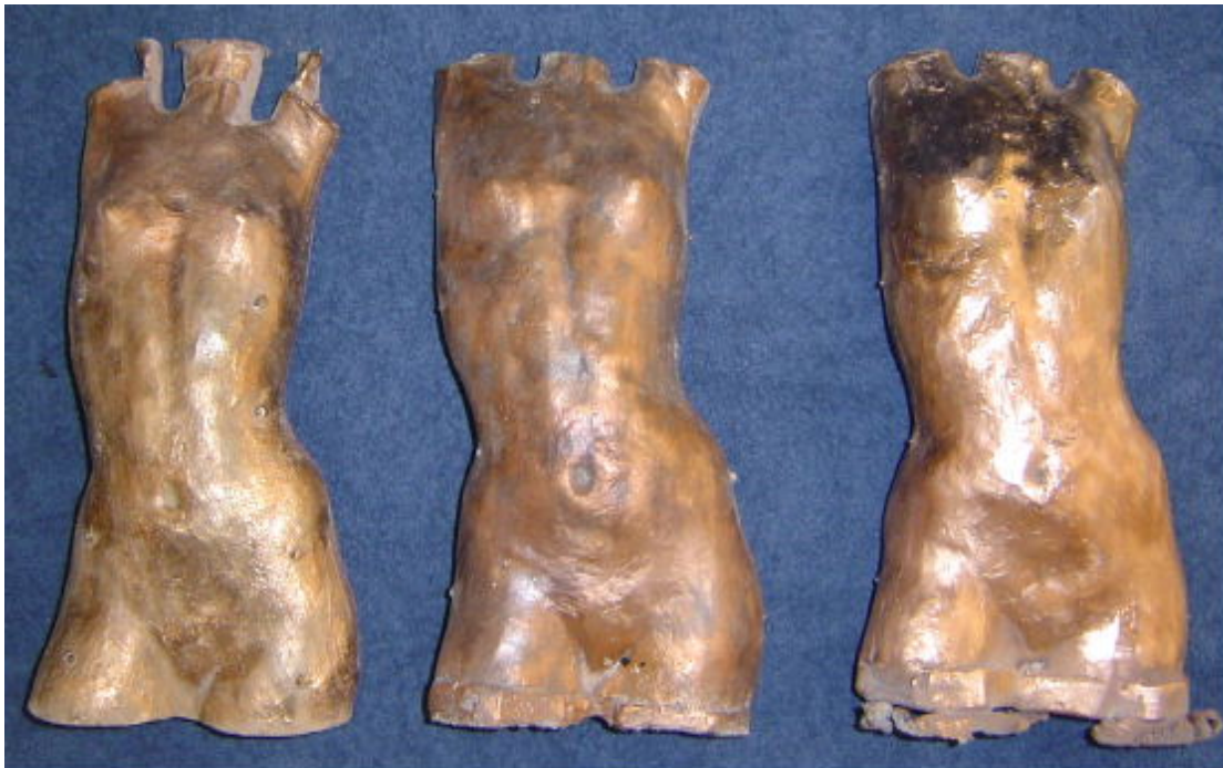
Figure 6.18 The three bronze female torsos (300 mm tall) whose cores were fired to 900 0 C, 945 0 C and 1000 0 C.
