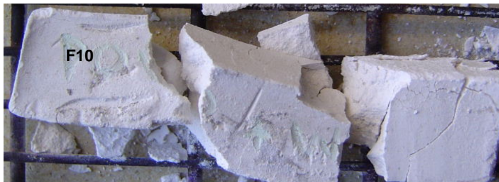
Figure 2.15 Formula F10 remains firm and soft after 72 hours and has not disintegrated into a powder.
