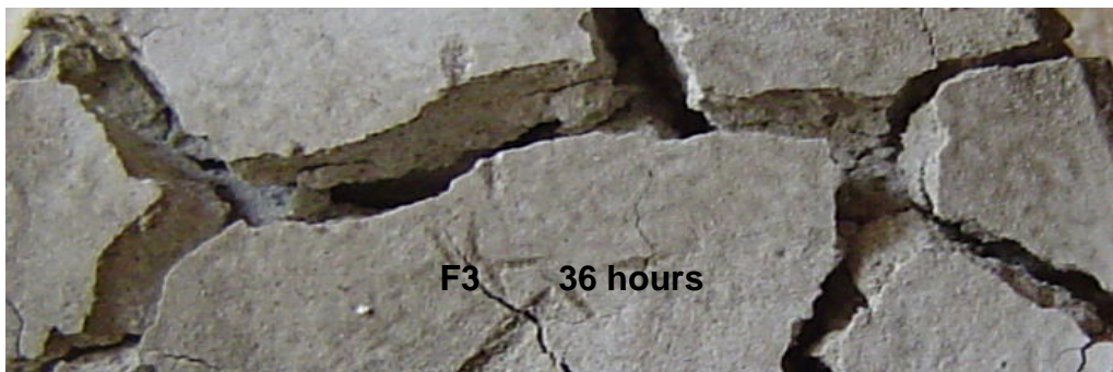
Figure 2.9 Formula F3 after 36 hours. The cracks have increased dramatically but the cracked sections remain as hard chunks (cf. table 2.1).
