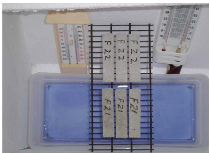
Figure 1.19 A photograph of a view looking down into the R H C apparatus which for illustration purposes has six sintered test bars placed on a metal grid above a trough of water
