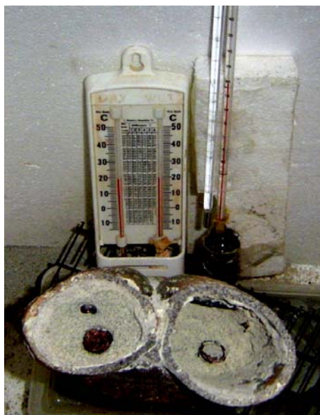
Figure 6.3 A photograph illustrating the bottom view of the 300 mm tall female torso bronze mould placed in the R H C apparatus on a metal grid which covers the water trough. A relative humidity instrument stands behind the bronze torso.
