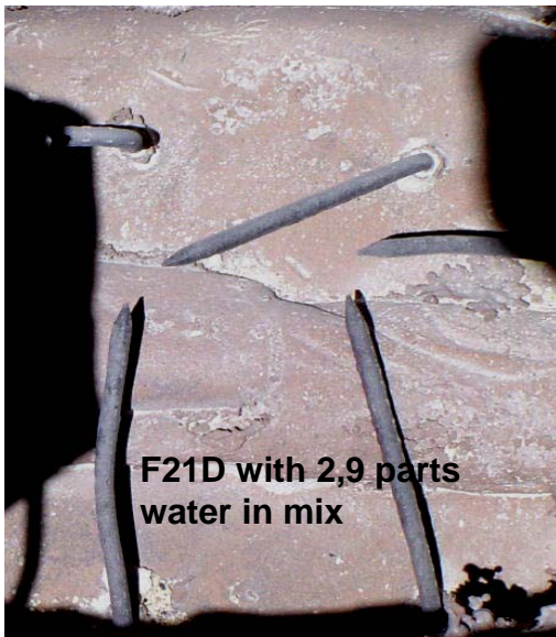
Figure 6.29 Internal view of figure 6.27
