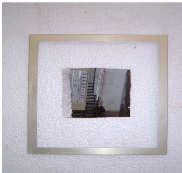
Figure 1.18 A photograph illustrating a view through the lid of the R H C apparatus. showing a maximum and minimum thermometer (relative humidity) as well as the wet and dry thermometers which are calibrated in half degree centigrade divisions.
