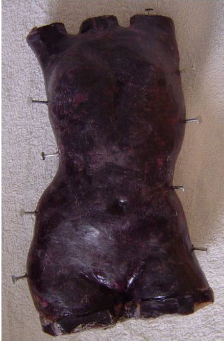
Figure 1.4 A photograph of the wax female torso that will be used to test various formulae in the fifth sub-problem. Note the core pins are in place.
