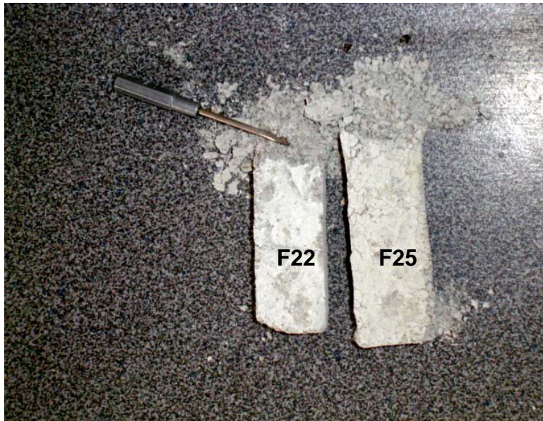
Figure 3.7 A photograph illustrating two partial disintegrated naked test bars made from formulae F22 and F25.
