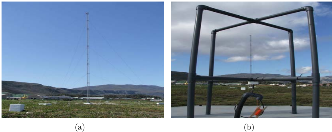
Figure 3.6: (a) Transmitter antenna and (b) Receiver antenna of the Hermanus ionosonde
