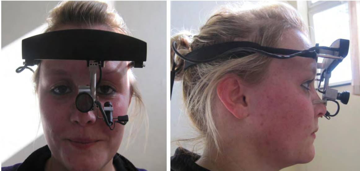
Figure 5: Subject fitted with the Dikablis eye tracking system.
