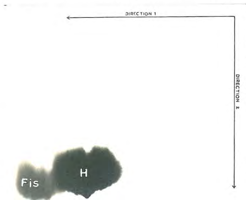
Fig. 4. Chromatogram of (+)-catechin band after adsorption separation of tubes 110-130, (Fig. 3). Fus = fustin.
