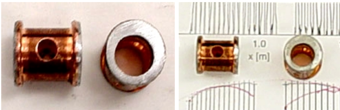
Fig.5.2.7 Lengthened tubes after soldering
