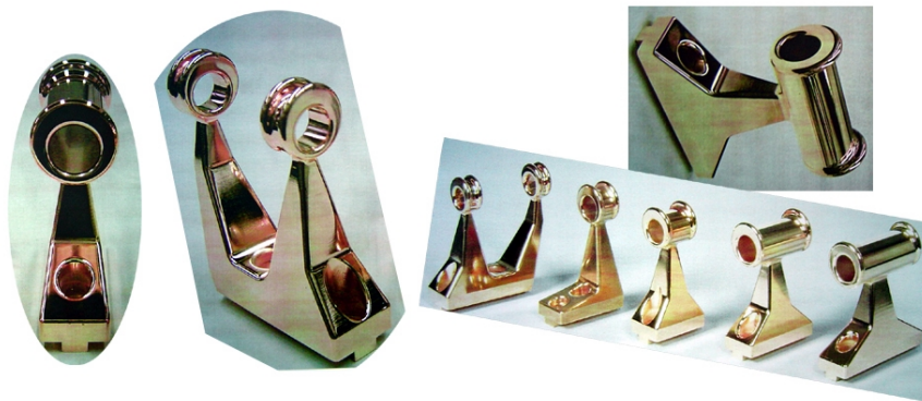
Fig.8.1 Some original drift tubes after copper plating
