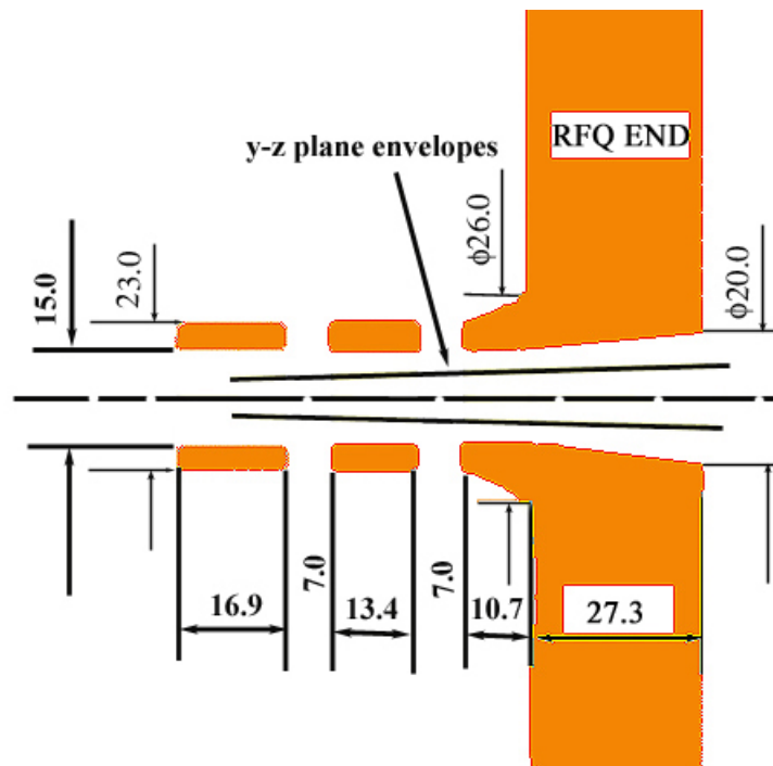
Fig.4.16 Buncher drift tube geometry (chamfer radius 1.5mm, tube thickness 4mm)
