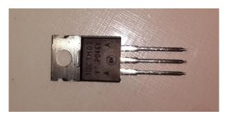
Figure 4-7: Selected rectifying diode D\_r for the MPPT power circuit
