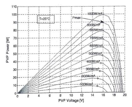
Figure 2-5: Simulated power/voltage curve characteristics of a PV panel (PVP) model at constant
