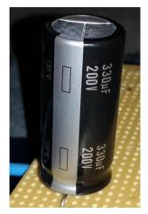
Figure 4-5: Selected capacitor C\_out for the MPPT power circuit
