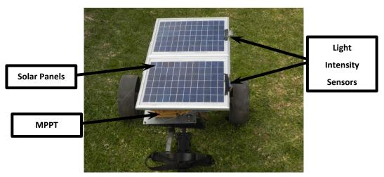
Figure 3-11: Final vehicle prototype
