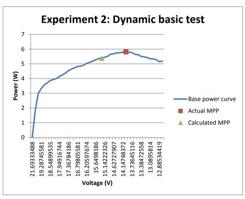
Figure 6-6: Base experimental power curve of while vehicle is in motion
