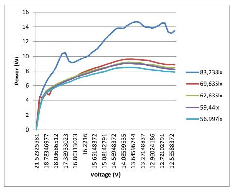
Figure 6-2: Power versus voltage for a range of 5 light intensities at constant 42°C
