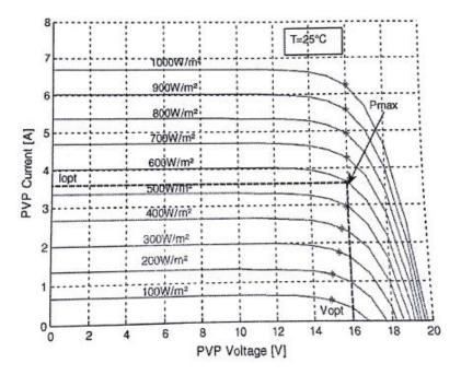
Figure 2-6: Simulated current/voltage curve characteristics of a PV panel (PVP) model at constant temperature (T) of 25°C [11]
