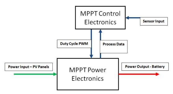
Figure 4-1: MPPT Functional Diagram
