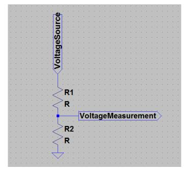
Figure 4-15 is a simple diagram of a universal voltage divider circuit.
