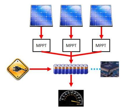
Figure 2-2: Energy flow schematic of a solar/electric vehicle
