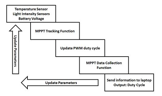
Figure 5-1: Schematic representation of MPPT controller
