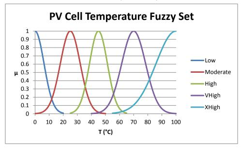
Figure 5-5: Gaussian membership functions for fuzzy set T\_pv
