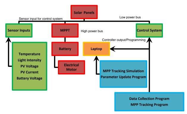
Figure 3-1: Experimental electrical and electronic system overview
