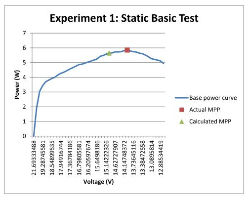
Figure 6-5: Base experimental power curve
