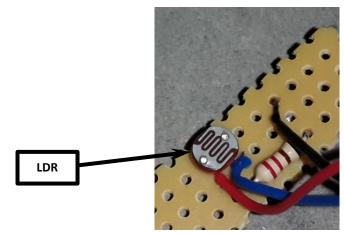
Figure 4-12 is an image of the selected light sensor.
