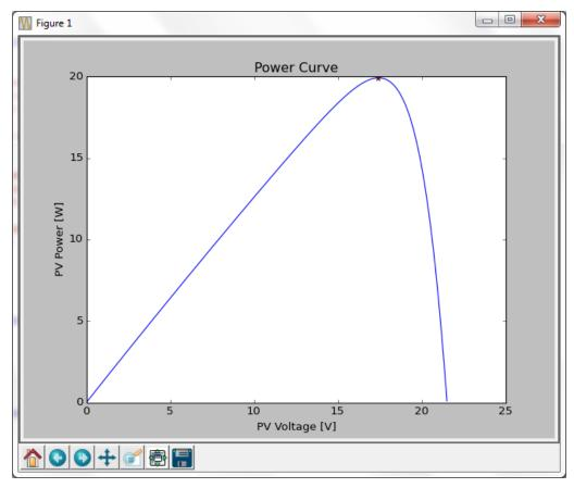
Figure 5-15: The power curve for the test PV panel as produced by the mathematical model at 25°C and 1000W/m2
