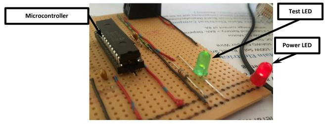
Figure 4-20: Basic microcontroller circuitry
