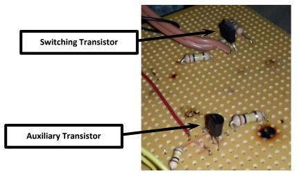
Figure 4-9: Transistor switching circuits
