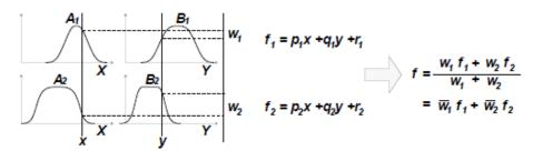
Figure 5-12: Example of the Takagi and Sugeno method for fuzzy inference [39]
