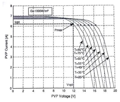
Figure 2-8: Simulated current/voltage curve characteristics of a PV panel (PVP) model at constant solar irradiation (G) of 1000W/m2 [11]
