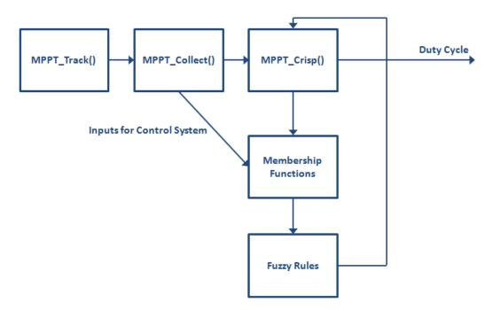
Figure 5-26: Functional flow diagram of MPPT tracking function
