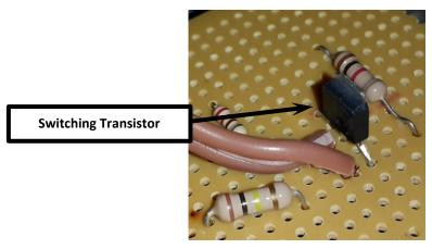
Figure 4-6: Selected switching transistor T\_s for the MPPT power circuit
