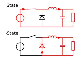
Figure 4-3: Circuit diagram illustrating the operation of a step-down DC-DC converter [24]
