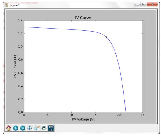
Figure 5-14: The I-V curve for the test PV panel as produced by the mathematical model at 25°C and
