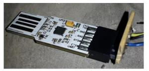
Figure 4-16: Selected UART to USB conversion module for serial communication
