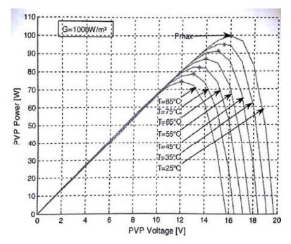
Figure 2-7: Simulated power/voltage curve characteristics of a PV panel (PVP) model at constant solar
