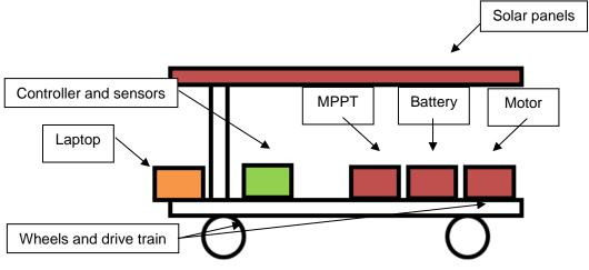
Figure 3-2 is a very basic diagrammatic concept of a solar vehicle.
