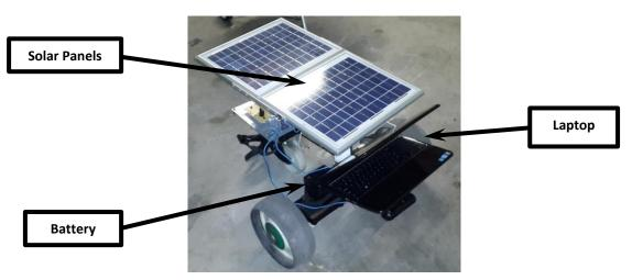
Figure 3-9: Solar panels mounted on the solar vehicle
