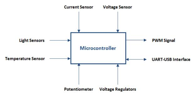
Figure 4-10: MPPT control circuit diagram
