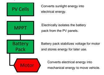
Figure 3-4: Basic flow diagram of solar vehicle electrical system
