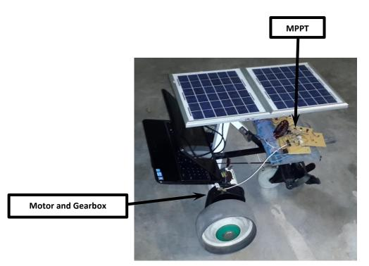
Figure 3-10: MPPT mounted on the vehicle
