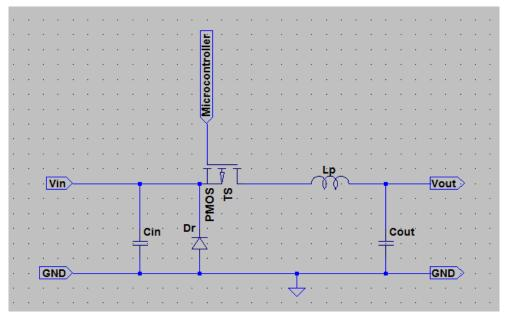
Figure 4-2: Step-down DC-DC converter circuit diagram
