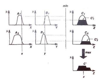
Figure 5-8: Illustration of the Mamdani method, using the Min-Max principle [34]
