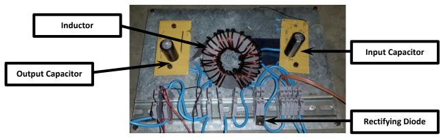
Figure 4-8: MPPT Power Electronics Circuit
