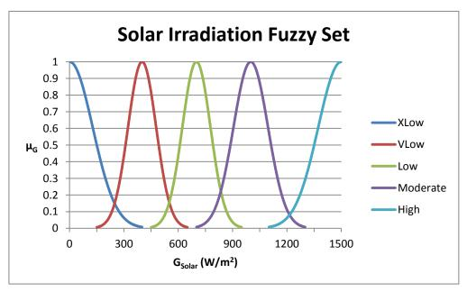
Figure 5-6: Gaussian membership functions for fuzzy set G\_solar
