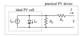
Figure 5-13: The representation of a PV cell as a semiconductor diode and current source
