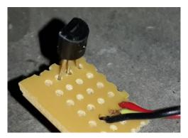
Figure 4-13: Temperature Sensor
