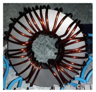
Figure 4-4: Manufactured inductor L\_p for the MPPT power circuit
