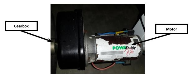
Figure 3-8: Gearbox assembly and motor of the electric golf trolley
