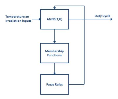
Figure 5-18: Functional diagram of simulated ANFIS controller
