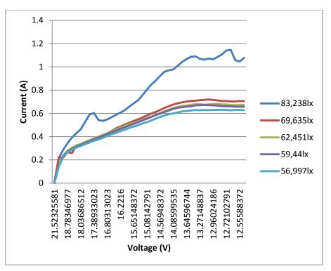
Figure 6-1: Current versus voltage for a range of 5 light intensities at constant 42°C
