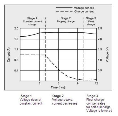
Figure 5-16: Charge curve of a lead-acid battery cell [42]
