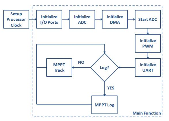
Figure 5-25: Functional flow diagram microprocessor software overview
