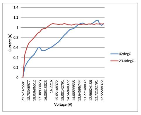
Figure 6-3: Current versus voltage for a range of 2 PV cell temperatures at constant light intensity
