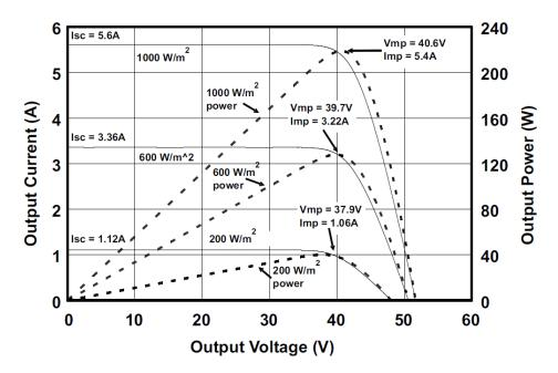
Figure 2-4: Example of a PV panel power curve [10]
