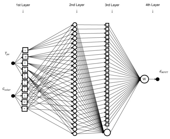
Figure 5-11 is an illustration of the proposed ANFIS controller.
