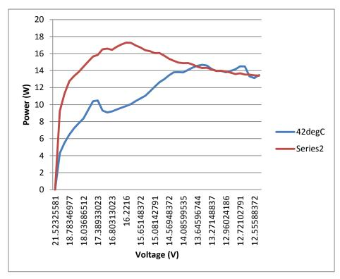
Figure 6-4: Power versus voltage for a range of 2 PV cell temperatures at constant light intensity
