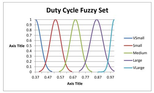
Figure 5-7: Gaussian membership functions for fuzzy set d\_MPPT
