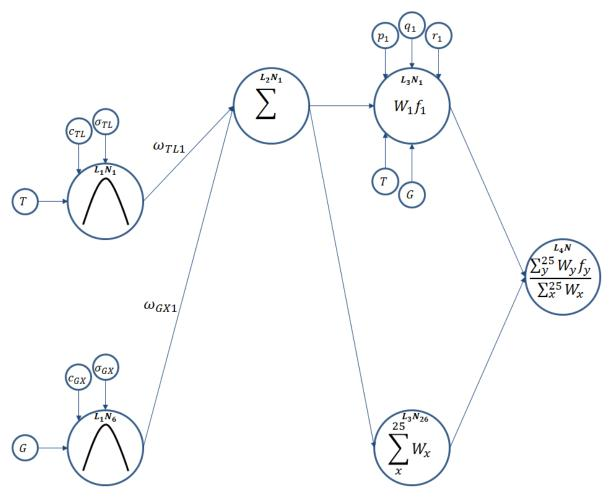
Figure 5-21: Section of the ANFIS algorithm
