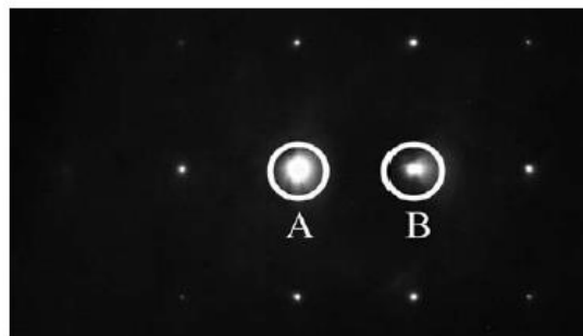
Figure 3.30: The location of the objective aperture (circles) on the SAED pattern when forming (A) BF and (B) DF images. (Williams and Carter 2009)
