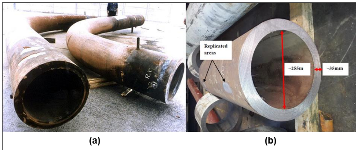
Figure 3.1: Images of (a) typical main steam pipes used at coal-fired power plants (Bohler) and (b) the X20 steel pipework used in this research (Molokwane 2014).
