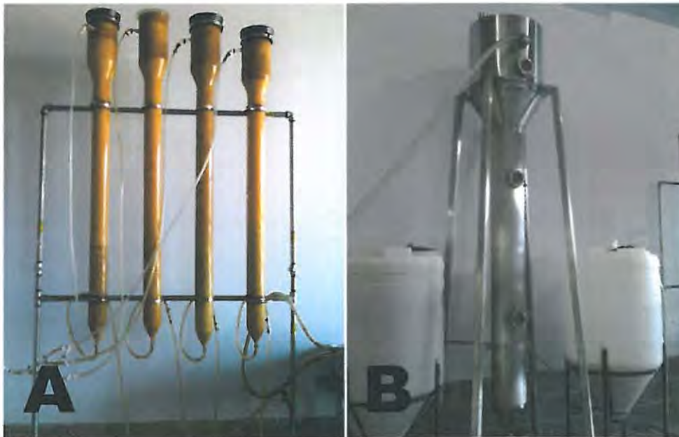
Figure 5.1 Photograph of the experimental apparatus; (A) pilot-scale PTBs, (B) commercial-Scale PTB.
