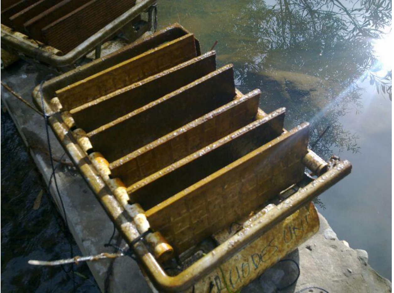
Plate 9. Grey clay tile substrate structure after its removal from the Kowie River following a 28 day incubation period. Photo by Tatenda Dalu
