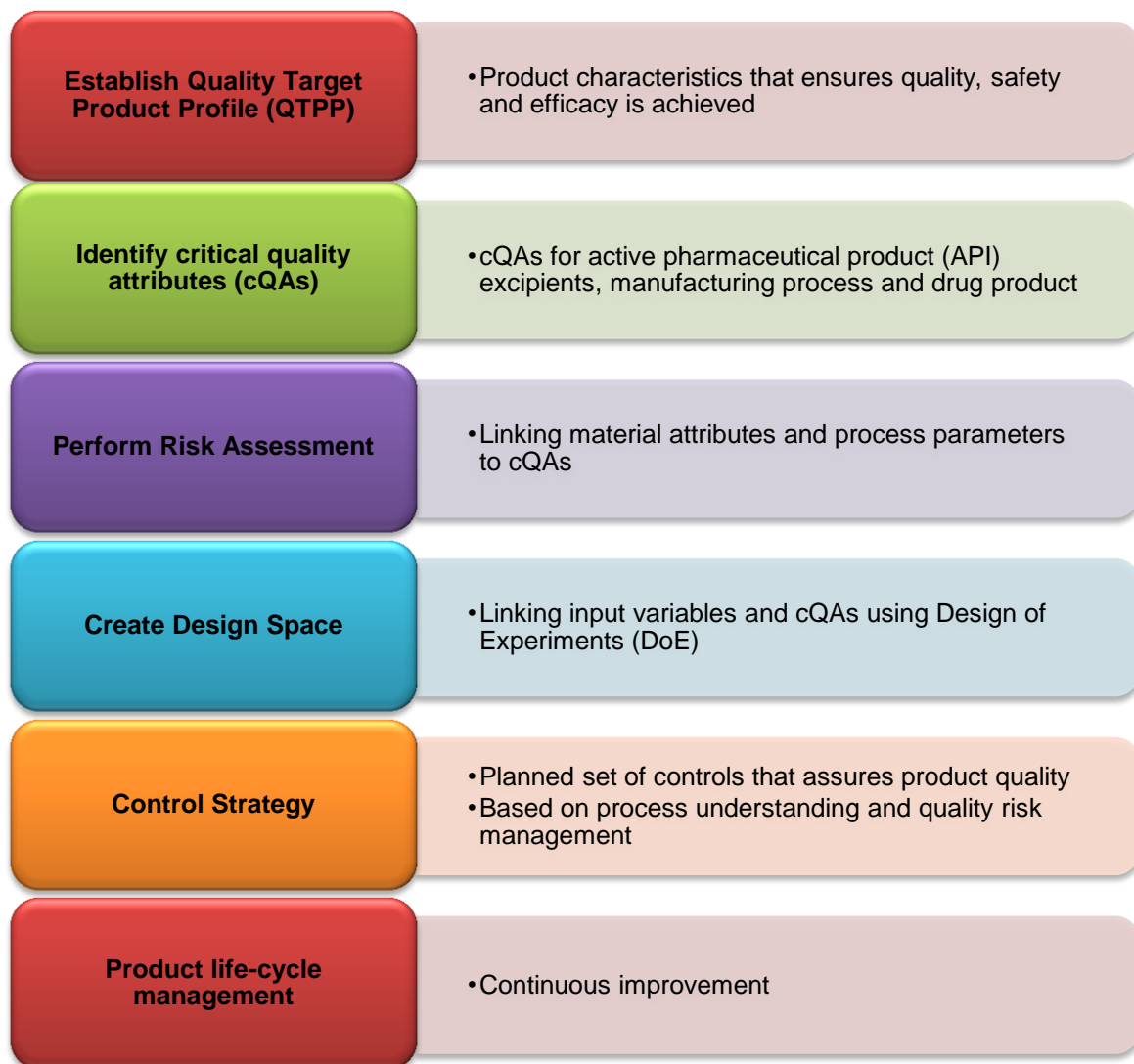
Figure 2.1 A flowchart illustrating the process of applying the principles of QbD (Adapted: Travedi, 2012)
