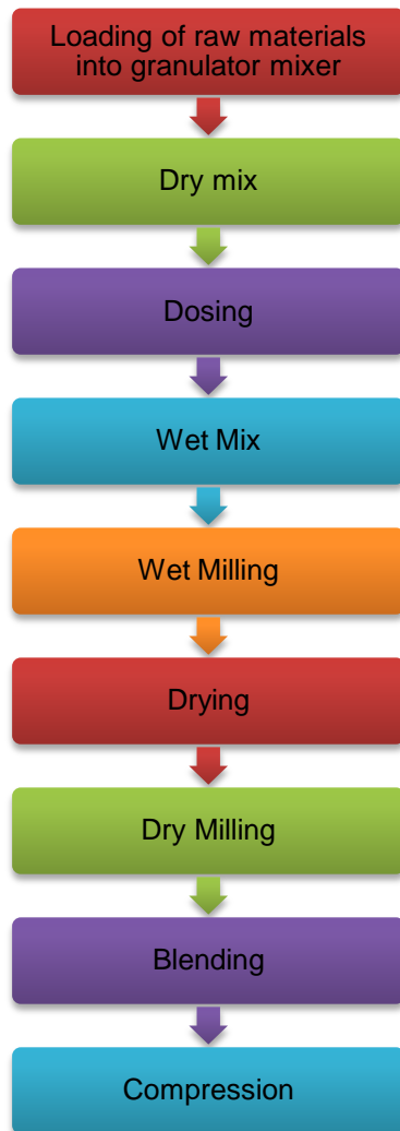
Figure 3.6 A flow diagram illustrating the process involved in the manufacturing of ethionamide 250 mg tablets
