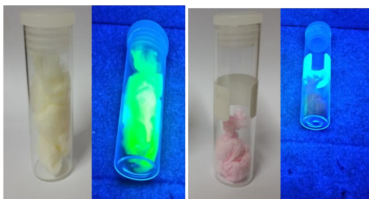
Figure 46: ( 1 ) (left) and ( 2 ) (right) BODIPY-PS nanofibers in ambient light and under UV irradiation.
