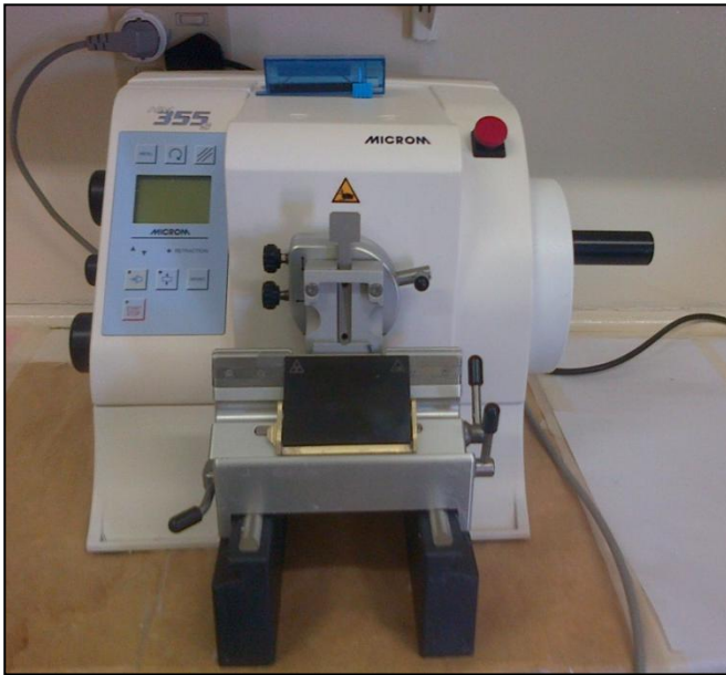
Figure 2.2 Rotary Microtome HM 355 S. Histology Laboratory, Walter Sisulu University
