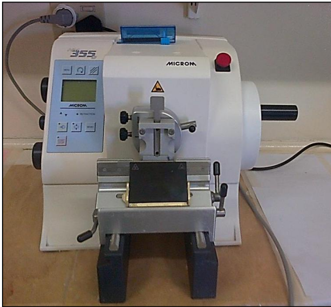
Figure 3.4 Rotary Microtome HM 355 S. Histology Laboratory, Walter Sisulu University.
