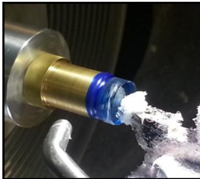
Figure 5.21 Chip build up on the diamond tool [55]
