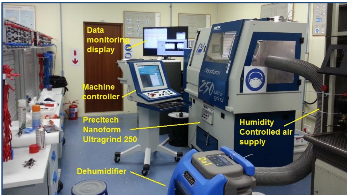
Figure 4.16 Setup for diamond turning of Contact lens polymer
