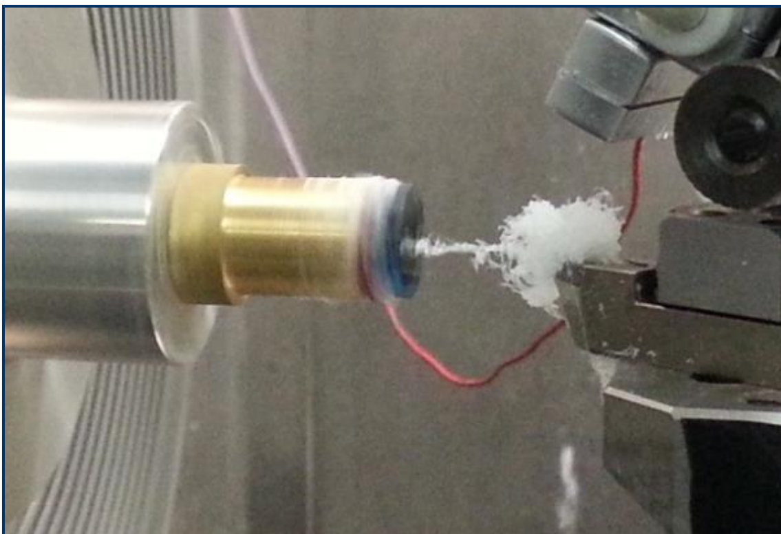
Figure 5.44 Strong triboelectric effects at very low humidity
