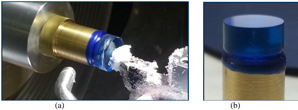
Figure 5.15 (a) Diamond machining of a contact lens button (b) top surface of mounted lens button
