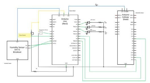
Figure 2: Wireless Node schema
