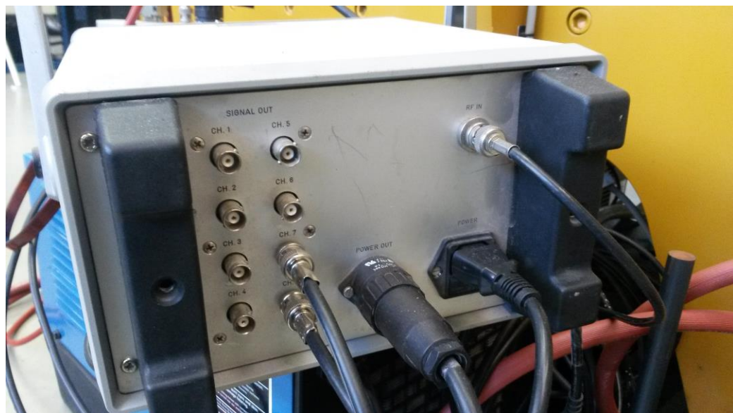
Figure 3.5. Demodulation unit rear
