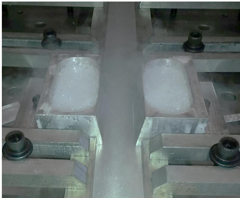
Figure 5.41. Dry ice and methanol heat sink
