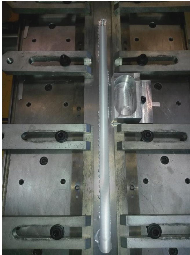
Figure 3.10. Bead on plate FSW
