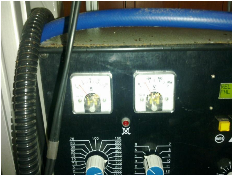
Figure 6.54 Portion of Alic-1 Control Panel Captured during EDM Process using Linear Actuator, Showing Stable Gap Voltage of 55V
