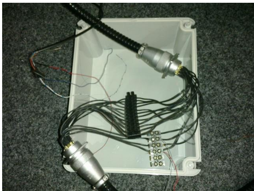
Figure 4.7 Alic-1 Servo Voltage Tapped Off at Connector Terminals
