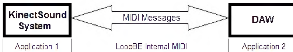
Figure 5.11 : Communication between the KinectSound system and the DAW using internal MIDI.
