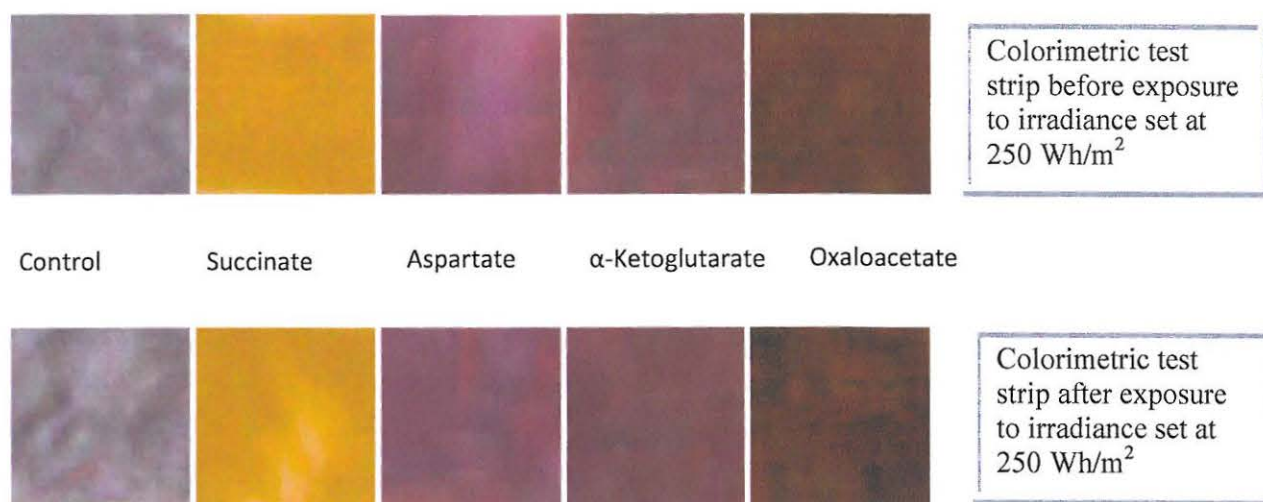
Figure 5.29: Photostability of the colorimetric probe. Photographs showing diazonium-nylon 6 probe strips before and after irradiance set at 250 Wh/m 2 upon exposure to succinate, aspartate, \alpha -ketoglutarate and oxaloacetate at 300 ng/ml and 120 sec exposure time for each substrate
