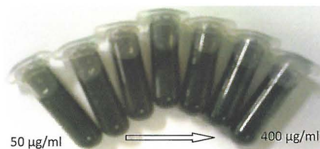
Figure 5.18: UV-Vis absorbance spectra and photograph showing colorimetric responses of various concentrations of oxaloacetate in phosphate buffer @ pH 7.4
