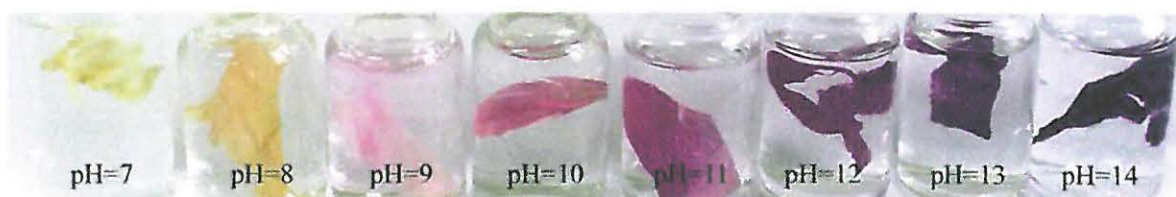
Figure 2.12: The colour change properties of pHS-NF membranes in different pH buffer solution. The pH sensitive membrane (pHS-M) showed a good mechanical integrity (Zhang et al., 2011b)
