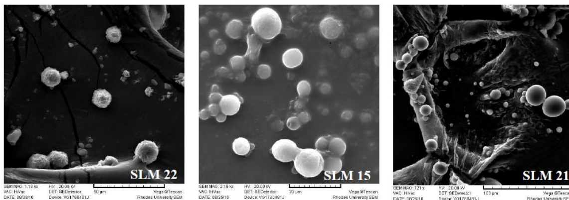
Figure 5.8 SEM images of KTZ-loaded SLM manufactured using different concentrations of KTZ: 3.3% w/v (SLM 22), 5% w/v (SLM 15) and 10% w/v (SLM 21) on the day of manufacture
