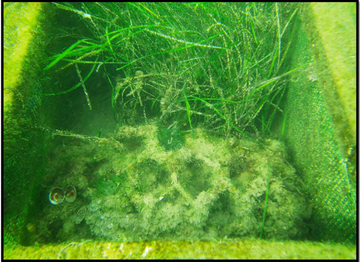
Figure 4.4. The choice chamber used in the choice experiment. Half of the choice chamber was covered in Z. capensis and the other half by a Reno mattress. In the photograph the matured Reno mattress structure is located in the forefront, and Z. capensis towards the back of the choice chamber.
