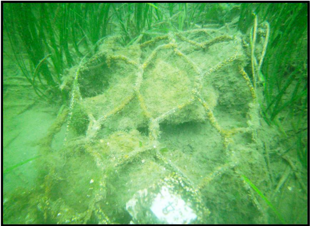
Figure 4.5. A matured Reno mattress sample used in the choice experiment.
