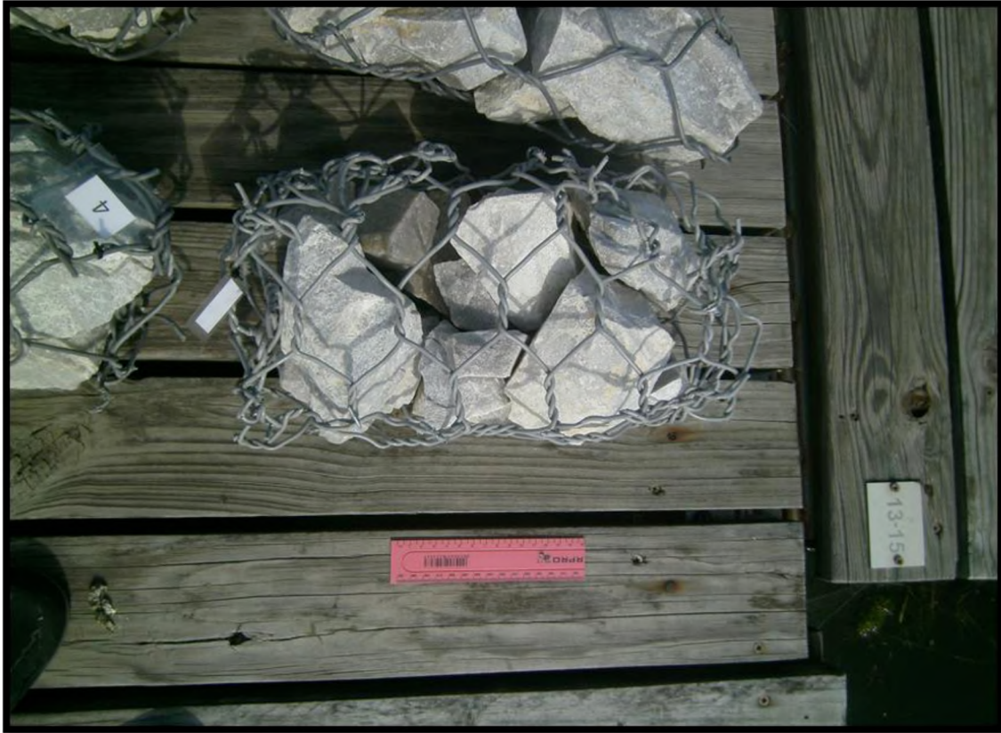
Figure 4.2. A sample Reno mattress structure used in the choice experiment conducted on H. capensis (ruler in picture = 15 cm).
