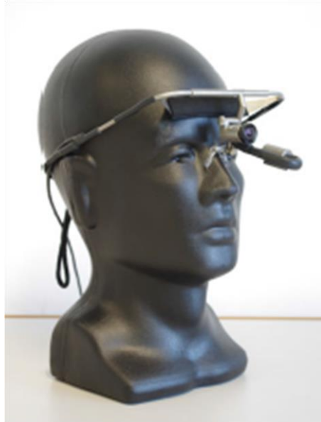
Figure 12: Doll fitted with the head unit of the Dikablis eye tracker (Louw, 2013, p. 55).
