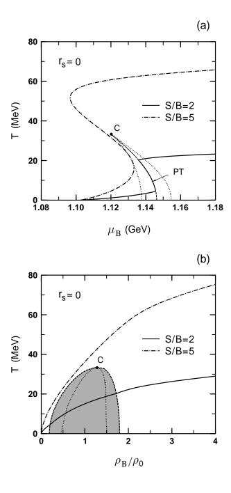
FIG. 9. Isentropes S/B = 2 (solid line) and S/B = 5 (dashed-dotted line) of quark matter with zero net strangeness. Lower (upper) part corresponds to the  $\mu_B - T$  ( $\rho_B - T$ ) plane. Dotted and dashed lines represent, respectively, spinodal and binodal boundaries of the two-phase region (shown by shading in the lower plot). Point C marks the critical point.
