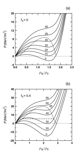
FIG. 6. Pressure isotherms for chemically equilibrated quark matter with  $r_s = 0$  (upper part) and  $r_s = 0.4$  (lower part). Temperatures are given in MeV near the corresponding curves. Boundaries of spinodal regions are shown by the dashed lines. The dashed-dotted line in lower plot shows the equilibrium pressure in the mixed phase-domain at T = 30 MeV.
