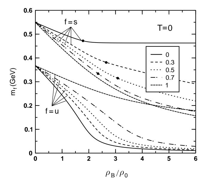
FIG. 2. Constituent masses of u and s quarks vs baryon density. Figures in the box show values of strangeness fraction  $r_s$ . Dots correspond to minima of energy per particle at given  $r_s$ .
