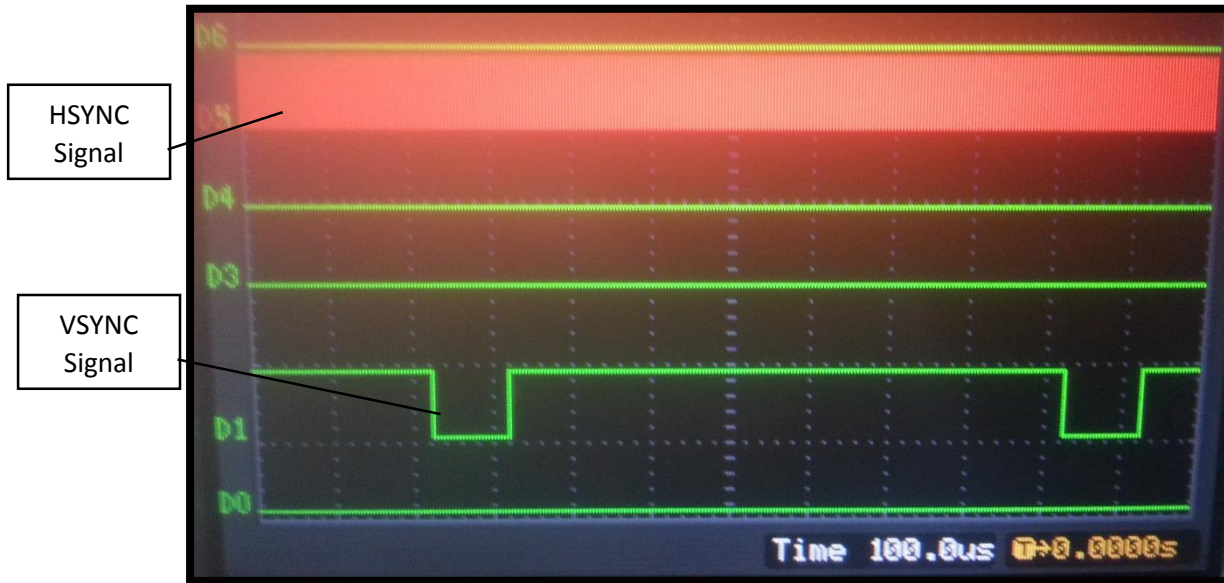
Figure 3.10 Oscilloscope digital signals of Vsync (bottom) and Hsync (top) signal
