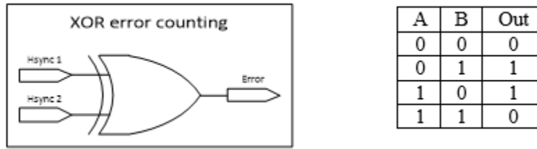
Figure 4.19 XOR schematic with truth table
