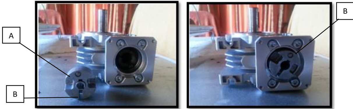
Figure 4.10 Worm gear drive with stepper motor connector
