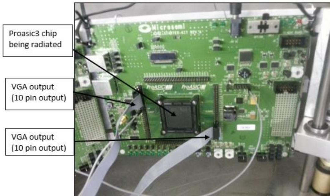
Figure 4.16 DUT that was radiated with 66MeV
