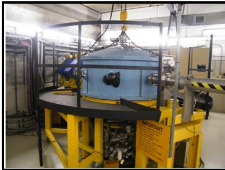
Figure 4.1 The A-Line scattering chamber at iThemba labs
