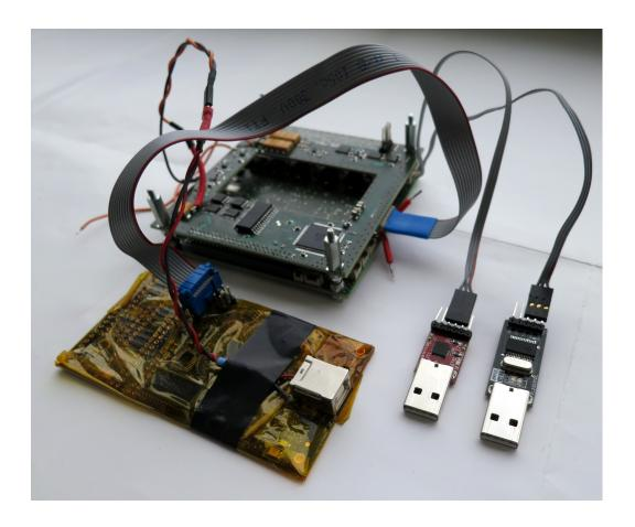
Figure 8: Table model with development kit. AVR Dragon on the left. Larger gray cable is JTAG cable, red & black wire is power lines from USB to MBP. Two USB-UART dongles are on the right. AVR Dragon is covered with tape to protect it from static electricity.
