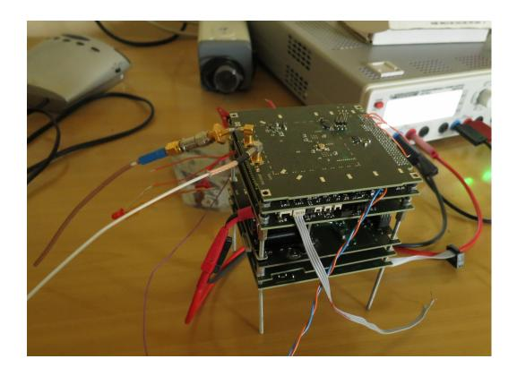
Figure 9: ESTCube-1 stack model in laboratory. Antennas are leaning to the left. Red and black wires are powering MPB from power supply unit. Orange wires for different debugging purposes are connected to Satellite System Bus.
