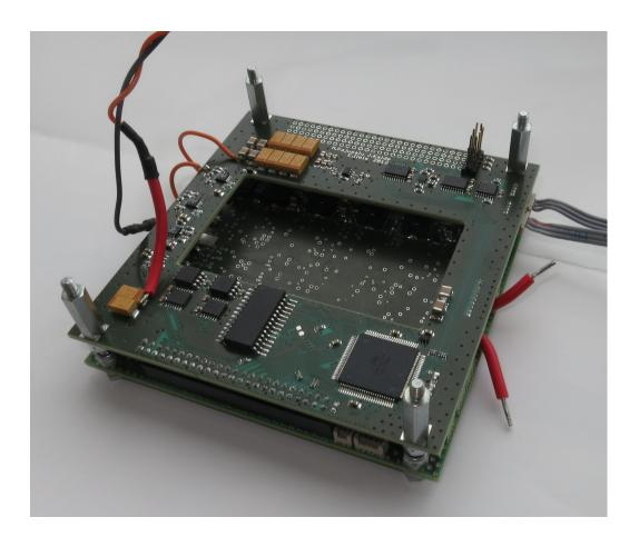
Figure 7: Table model for EPS development. Atmega1280 is seen in the lower right corner. Hole in the center is absence of batteries.
