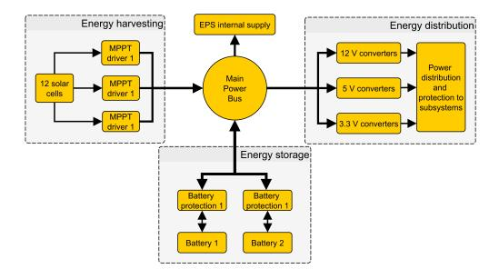
Figure 1: General design of the electrical power system
