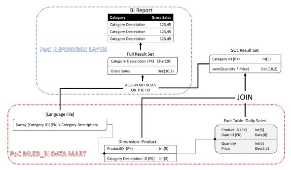
Figure 5-4: PoC physical level design for BI report delivery
