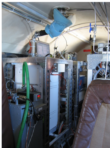
Figure 11: The NAIS (the box instrument in light grey inside the rack) with connection to the sample air inlet on the top inside the Falcon aircraft.
