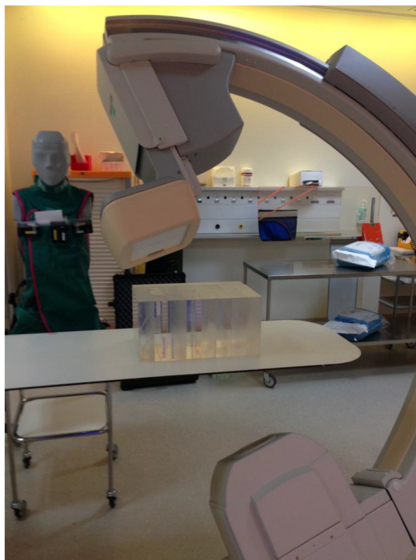
Figure 3. Set-up of anthropomorphic phantom in angiography room.
