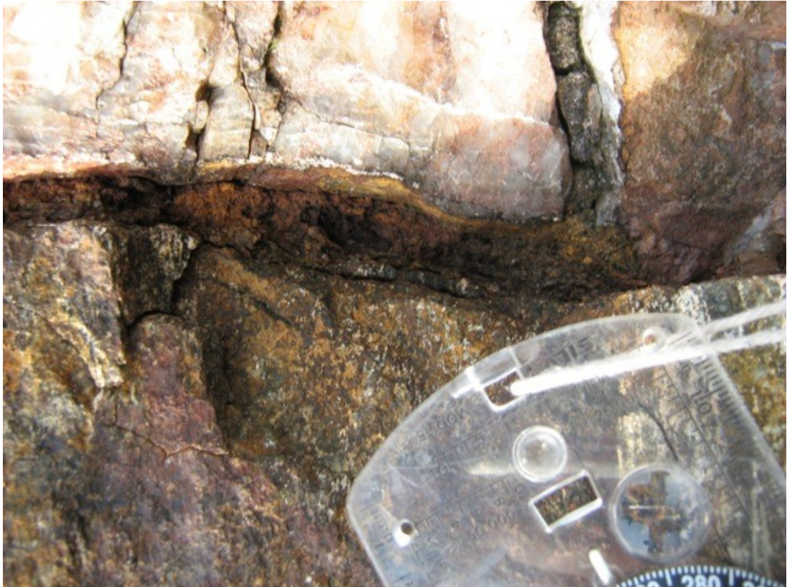
Gouge along the margin between a quartz-pyrite vein and the Lewisian country rock (NC 0855, 3102).
