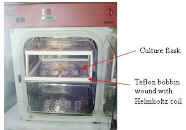
Figure 7. Magnetic field exposure facility fabricated using Teflon frame wound with Helmholtz coil housed inside the \text{CO}_2 incubator for studies on cellular models.
