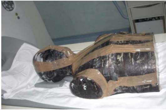
Fig. 1 Photograph of the RANDOs anthropomorphic phantom in the Siemens Definition Edge 128-slice CT scanner
