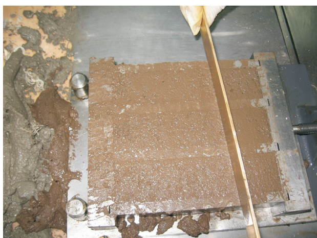
Fig. 5 – Filling of standard three-prism mould.
