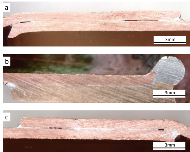
Figure 4 Defects of soldered joints a) incomplete running-in of solder b) running-out of solder, c) voids in capillary clearance
