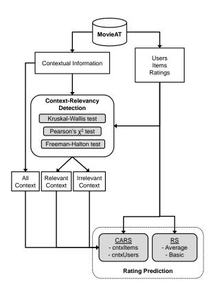
Fig. 1. Experimental design. The experiment was conducted on the data from the MovieAT database. Three statistical tests were used for the context-relevancy detection, and four models were used for the ratings prediction.
