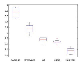
Fig. 5. Boxplot of the results for the CARS-cntxUsers model. Vertical axis shows the RMSE value. These results are obtained by the 10-fold cross validation for the Average and Basic models, and CARS-cntxUsers model using All, Relevant and Irrelevant contextual information.
