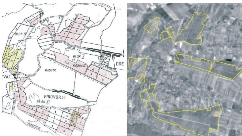
Fig. 2. and 3. Importing and assessment of old sketches and maps into GIS. Left: An example of an old plan; Right: The map of plots can be represented in a satellite image after geo-referencing.
