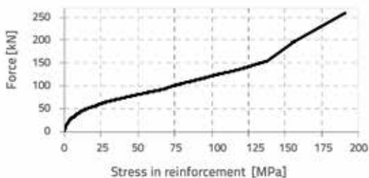
Figure 11. Diagram showing dependence between stress in reinforcement and concentrated force F
